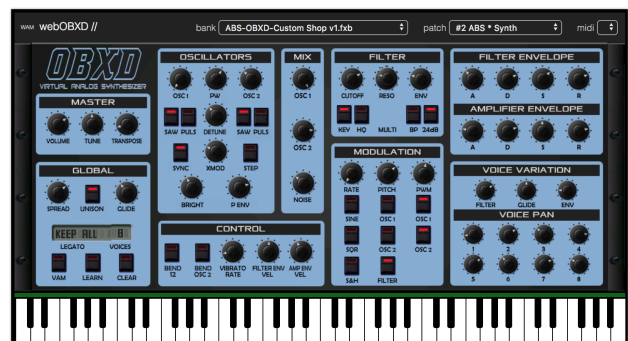
Figure 13. OBXd Oberheim emulation, originally written in C++ and ported to WebAssembly by webaudiomodules.org.
