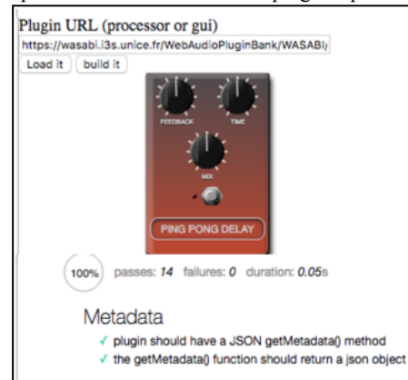
Figure 12. Online plugin tester: enter the plugin URL to validate the plugin before publishing to a repository.
