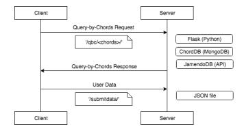
Figure 1: Architecture of the system.
