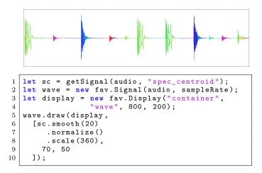
Figure 2: Waveform coloring with Spectral Centroid
