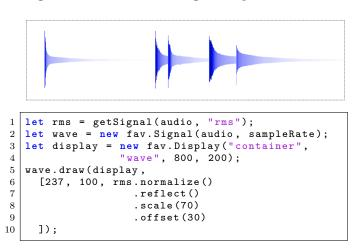
Figure 3: Waveform luminance coloring using RMS
